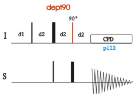
The time intervals depicted in the pulse sequence diagrams are not drawn to scale. For example, d1 is typically a few seconds while p1 is typically a few microseconds in length.
