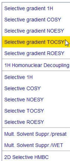
The default parameters are taken from the standard parameter set SELMLGP. If desired, click **Change Shape** to modify the **Gaus1\_180r.1000** pulse. A mixing time of **0.06 s** to **0.08 s** is typical for the TOCSY experiment.
