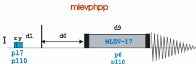
The time intervals depicted in the pulse sequence diagrams are not drawn to scale. For example, **d1** is typically a few seconds while **p1** is typically a few microseconds in length.
