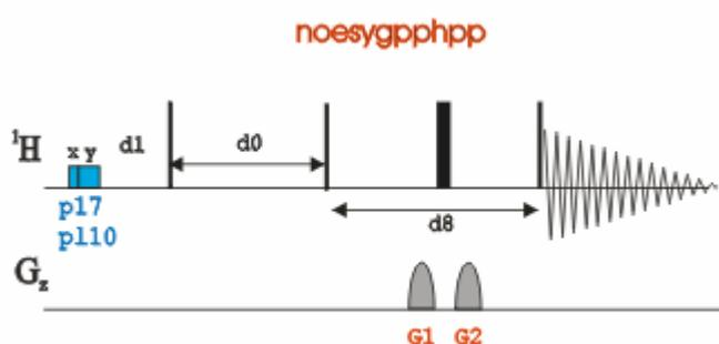
The time intervals depicted in the pulse sequence diagrams are not drawn to scale. For example,  $d_1$  is typically a few seconds while  $p_1$  is typically a few microseconds in length.
