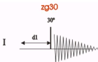
The time intervals depicted in the pulse sequence diagrams are not drawn to scale. For example, d1 is typically a few seconds while p1 is typically a few microseconds in length.
