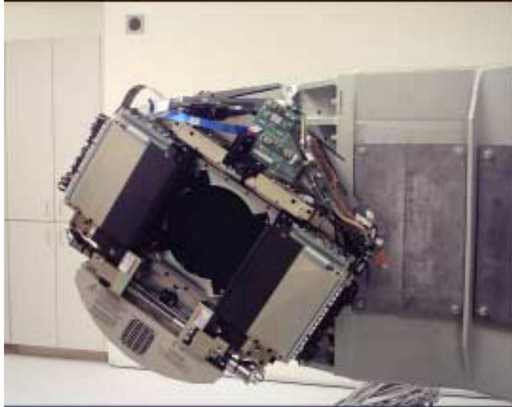
View of the Collimators (Jaws) and MLCs in the Treatment Head
