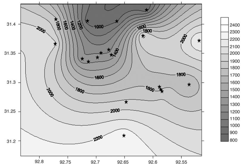
Figure 5. The depth of the base of brackish water from the earth's surface for the Hot Wells area ranges from about 800 ft to 2200 ft. This is the depth to the top of the first sand fully saturated with water that has a dissolved solids concentration over 10,000 ppm. The stars on the figure are the 21 wells drilled deep enough in the Hot Wells study area to reach the base of brackish water.
