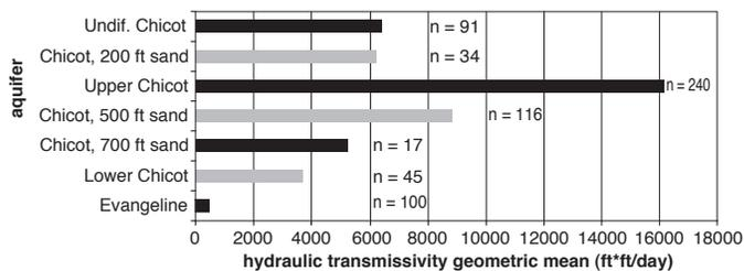
Figure 9. Transmissivity values of major aquifers in southwestern Louisiana. This region’s 707 transmissivity values have been determined from analysis of U.S. Geological Survey (2003) specific capacity data by using the Bradbury and Rothschild (1985) technique.
