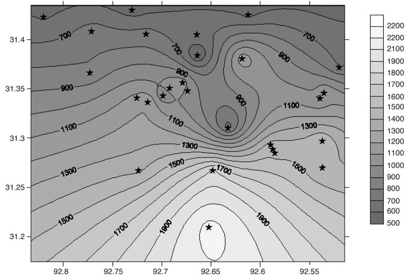
Figure 4. The depth of the base of freshwater from the earth's surface for the Hot Wells area ranges from about 500 ft to 2000 ft. This is the depth to the top of the first sand fully saturated with water that has a dissolved solids concentration over 1,000 ppm. The stars on the figure are the 30 wells drilled deep enough in
