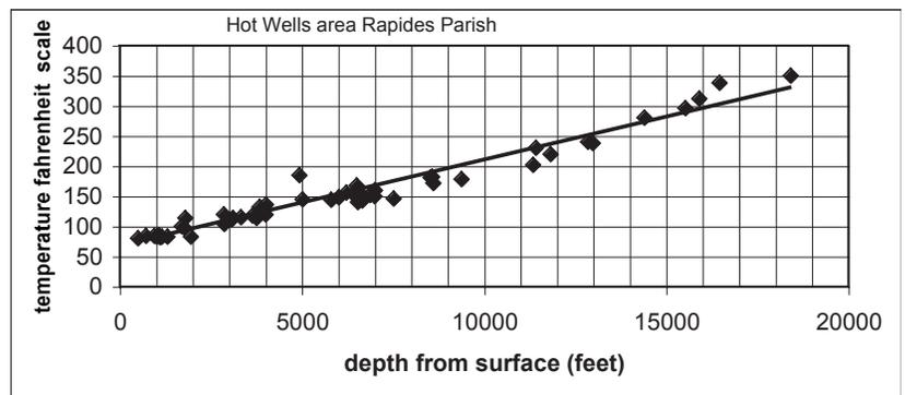
Figure 2. The 54 temperature results observed from 38 wells in the Hot Wells study area fall generally in a straight line. The increase of temperature with depth is 1.42°F/100 ft. The temperature at the surface is 66°F. The regression coefficient is 0.957 which means over 95% of temperature variation can be explained by a linear regression function displayed by the straight line.
