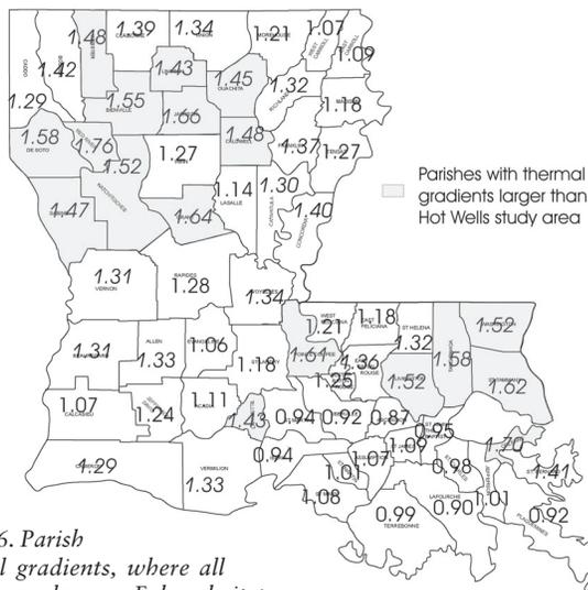
Figure 6. Parish thermal gradients, where all values are degrees Fahrenheit per 100 feet downwards. Parishes that have thermal gradients larger than the state average are in italics, while parishes with thermal gradients smaller than the state average are in block text.
