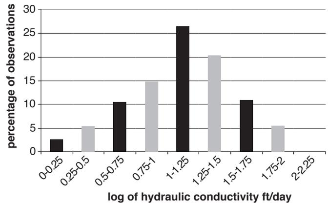
Figure 1. The Sparta Aquifer of northern Louisiana is typical of sand aquifers in that the distribution of hydraulic conductivity values of this unit is log normally distributed.
